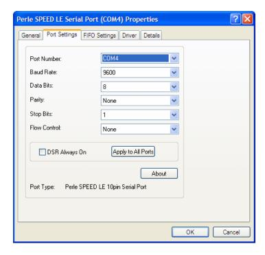
8. In the Port Settings page, set the **Port Number**, **Baud Rate**, and any other configuration parameters you require.
